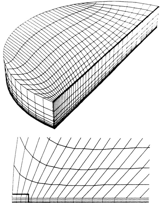
Figure 5. The three-dimensional mesh of one quarter of the SNL-CA combustion chamber. A blow up of the corner where the injection occurs is shown in the lower figure. The box in the corner of this figure is the size of the mesh used in the simulations shown in Figs. 2-4.
