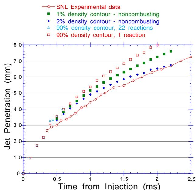
Figure 8. Comparison of the penetration history of the hydrogen jet of the KIVA simulation and the SNL-CA experiments. The penetration for the combusting KIVA simulations is presented for the maximum axial extent of the 90% total density contours. The penetration for the noncombusting simulation is as in Fig. 6.
