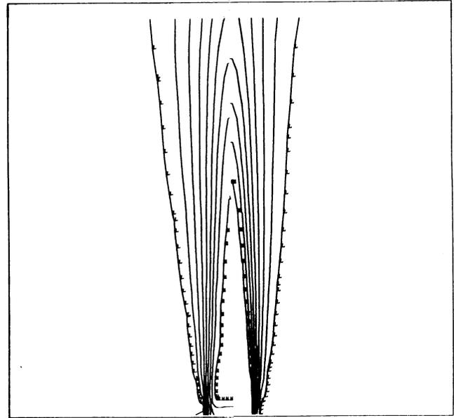
Figure 3. Mach number (left) and hydrogen mass fraction (right) contour plot for the 2D injection simulation near the orifice. The contour range for the Mach number is from 0.12 (marked L) to 1.1 (marked H) with intervals of 0.123. The contour range for the mass fraction is from 0.10 to 0.90 with intervals of 0.01.
