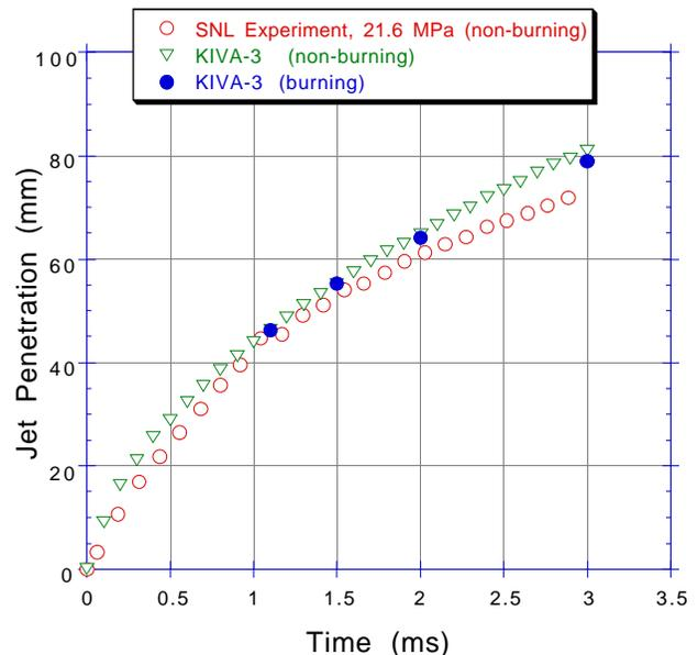
Figure 7. Comparison of the penetration history of the methane jet of the KIVA simulation and the SNL-CA experiments. The penetration in the KIVA simulations is based on the 1% methane density contours. A similar plot of data using 2% contours falls exactly on top of the data at late times.
