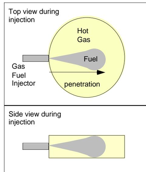
Figure 1. Schematic of the combustion bomb for fuel injection experiments.
