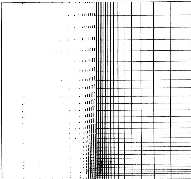
Figure 2. Velocity vector field and mesh for the 2D injection simulation near the orifice.
