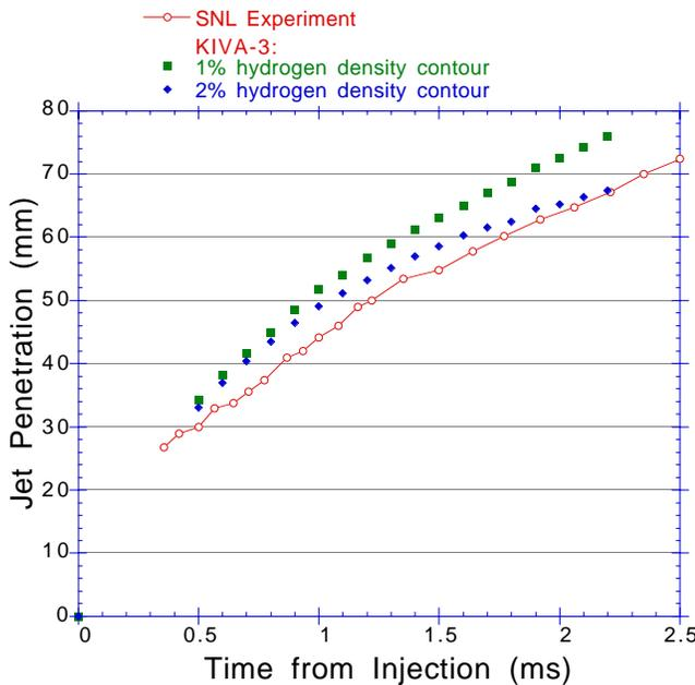
Figure 6. Comparison of the penetration history of the hydrogen jet of the KIVA simulation and the SNL-CA experiments. The penetration in the KIVA simulations is presented for the maximum axial extent of the one and two percent hydrogen density contours.
